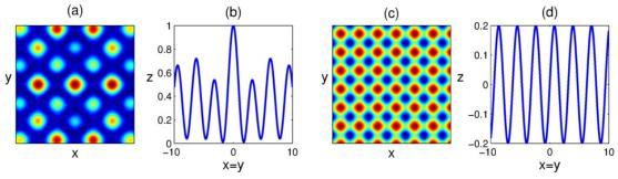
Figure 3.5 : (a) Real part, (b) Cross section of the real part, (c) Imaginary part, (d) Cross section of the imaginary part of the potential in Eq. (3.18) with  $V_0 = 0.04$  and  $W_0 = 0.1$ .
