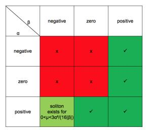
**Figure 6.1** : Existence of analytical solutions of the (1+1)D CQNLS equation without any potential.
