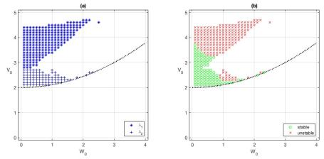
**Figure 7.8**: (a) Numerically obtained solitons for  $\alpha = -1$ ,  $\beta = 1$  and varying potential depths, (b) Analytically obtained, nonlinearly stable (marked as green circles) and nonlinearly unstable (marked as red crosses) solitons.
