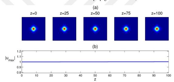
Figure 7.10 : (a) Nonlinear evolution of the numerically obtained soliton for  $V_0 = 3$ ,  $W_0 = 0.1$  and  $\alpha = \beta = -1$  (view from top), (b) Maximum amplitude as a function of the propagation distance *z*.
