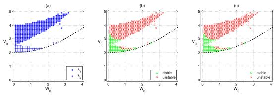
**Figure 6.7** : Numerically obtained solitons of the (1+1)D CQNLS equation with a  $\mathscr{PT}$ -symmetric potential for varying potential depths in the self-defocusing cubic, self-focusing quintic case ( $\alpha = -1$ ,  $\beta = 1$ ), (b) Numerically obtained, nonlinearly stable (marked as green circles) and nonlinearly unstable (marked as red crosses) solitons, (c) Analytically obtained, nonlinearly stable (marked as green circles) and nonlinearly unstable (marked as red crosses) solitons.
