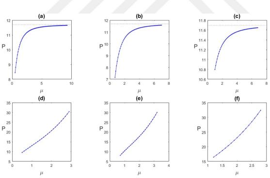
Figure 8.5 : Power as a function of propagation constant for the numerically obtained solitons: (a) s = 0, no defect; (b) s = 0, positive defect; (c) s = 0, negative defect; (d) s = 0.1, no defect; (e) s = 0.1, positive defect; (f) s = 0.1, negative defect.
