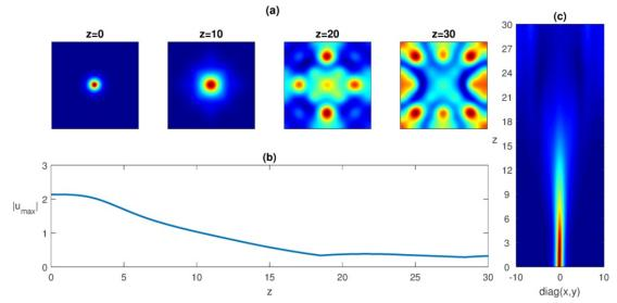
**Figure 8.3** : Nonlinear evolution of the soliton obtained for s = 0,  $\mu = 1.1$  and with a  $\mathcal{PT}$ -symmetric potential with negative defect: (a, c) View from top, (b) Maximum amplitude as a function of the propagation distance *z*.
