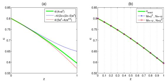
Figure 5.1 : Exact solution of the equation  $u_z = u^2 - u$  in comparison with the numerical solutions obtained by means of split-step method using Strang splitting with step size (a) h = 1 and (b) h = 0.1.
