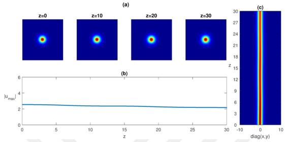
Figure 8.4 : Nonlinear evolution of the soliton obtained for s = 0.2, μ = 1.1 and with a *PT*-symmetric potential with negative defect: (a, c) View from top, (b) Maximum amplitude as a function of the propagation distance z.
