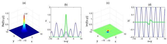
Figure 7.14 : (a) Real part, (b) Cross section of the real part, (c) Imaginary part, (d) Cross section of the imaginary part of the obtained soliton with  $V_0 = 1$ on the lattice with negative defect.
