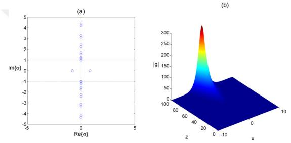
**Figure 6.13** : (a) Linear spectrum of the analytically obtained soliton of the (1+1)D CQNLS equation with a  $\mathcal{PT}$ -symmetric potential for  $V_0 = 3.6$  and  $W_0 = 0.1$  in the self-defocusing cubic, self-focusing quintic case  $(\alpha = -1, \beta = 1)$ , (b) Linear evolution of the soliton.
